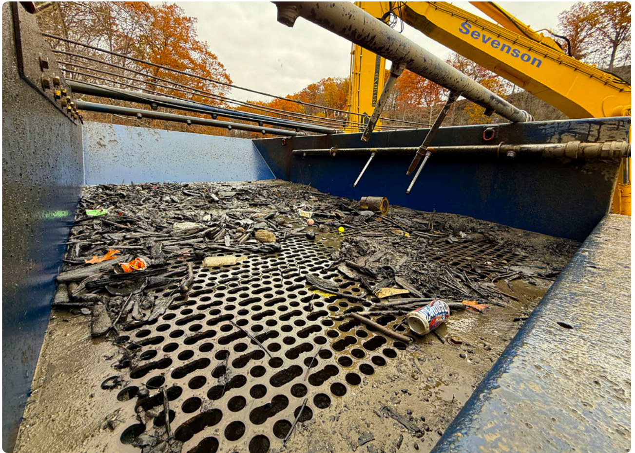
Larger debris is separated out from the sediment during dredging using screens that catch the material.
